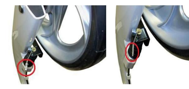
• Loosen the cable fastener with a 4mm Allen wrench and remove.
