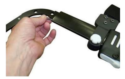
• Using a long needle nose pliers grasp the brake cable through the cable hole and pull the cable out of the frame.
