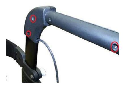
• Pull up on the cable and guide it through the hole in the lower frame. Continue pulling until it is out of the frame. Make sure the cord is not pulled into the frame.
