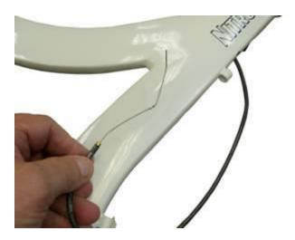
• Tape a 5' length of cord to as much or the brake cable as possible. Do not tape the cord to the cable housing. Do not make the taped section wider then the cable housing.
