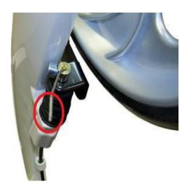
• Loosen the cable fastener with a 4mm Allen wrench and remove.
