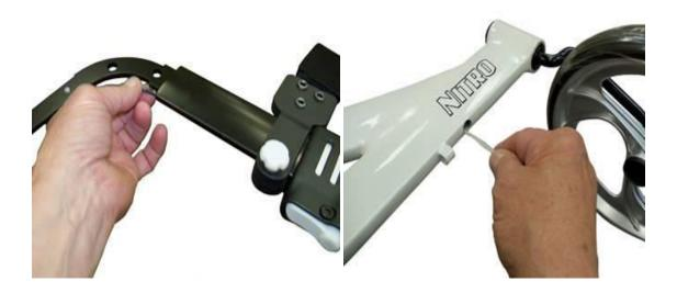
• Remove the cord from the old brake and tape the cord to the cable of the new brake. Do not tape the cord to the cable housing. Do not make the taped section wider then the cable housing.
