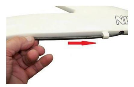
• Use the cable adjuster to make any needed adjustments to the brake. If the brake can not be adjusted to engage the wheel, loosen the cable faster and reposition as needed.
