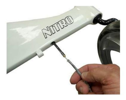
• Attach the handle bar housing back onto the frame. The largest of the three screws goes into the center hole.
