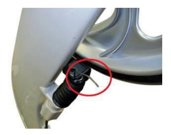
• Remove the brake cable from the cable adjuster and spring.
