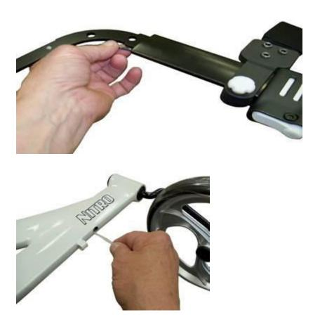
• Push the new brake cable down until the brake cable can be seen in the cable hole in the bottom of the frame.
