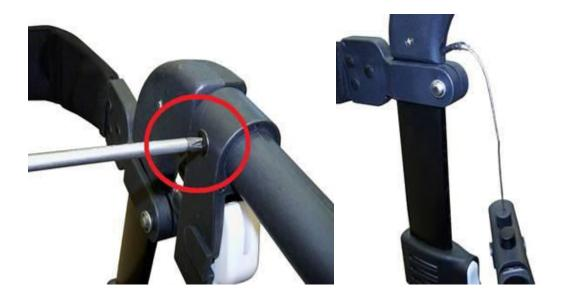
• Remove the three screws holding the handle bar housing to the handle bar frame using a Phillips screw driver. Separate the two half's of the brake handle to remove them from the hand bar.
