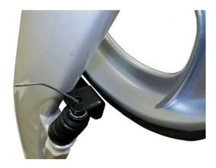
• Slide the cable fastener on to the cable until the brake blade is about 1/8" from the wheel.
