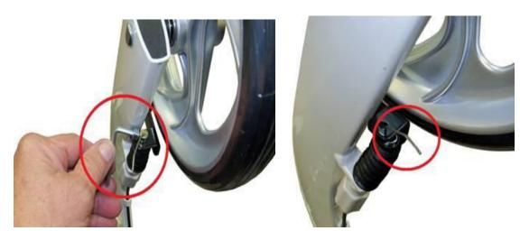
• Remove the brake cable from the cable adjuster and spring.
