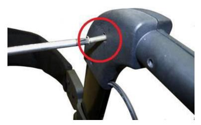
• Slide the brake handle on to the handle housing. As the brake is slide forward pull on the brake cable coming out of the lower frame. Screw the brake handle in place.
