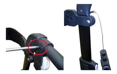
• Remove the three screws holding the handle bar housing to the handle bar frame using a Phillips screw driver. Separate the two half's of the brake handle to remove them from the hand bar.
