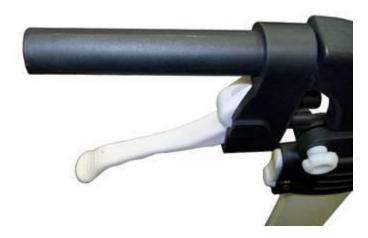
• Remove the screw holding the brake handle onto the handle bar using a Phillips screw driver. Remove the brake handle.
