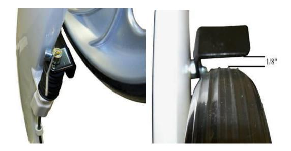
• Tighten the cable fastener.
