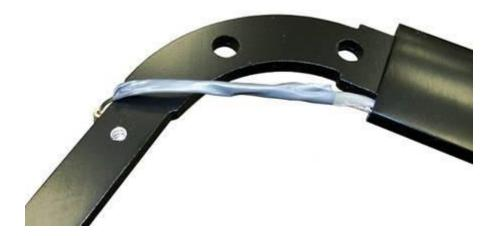
• Pull the cord until the brake cable comes through the bottom of the frame.
