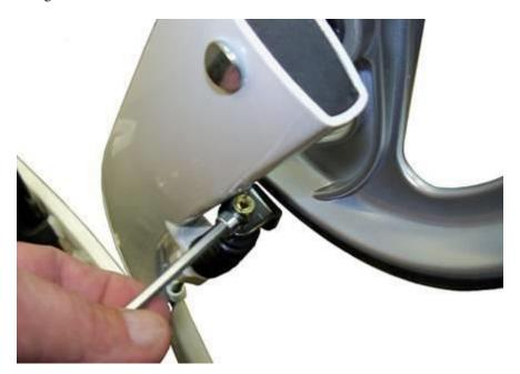
• Push any excess brake cable in to the hole in the lower frame.
